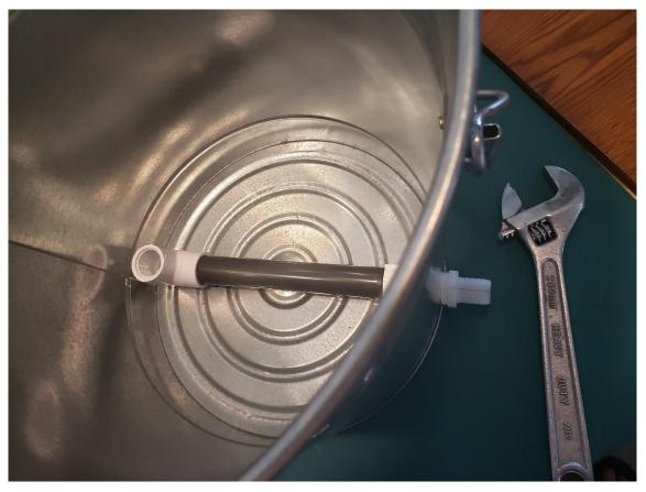
11. Screw the riser into the lower section.
