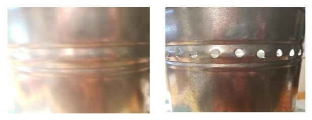
13. Then test it – attaching  $\frac{3}{2}$  flexible tubing to pump and then to outside barb fitting on bucket. If you are lucky you won't have to drill more holes  $\bigcirc$
